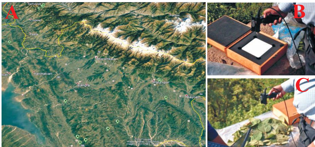
Fig. 5 A) Locations surveyed for spectral data collection (highlighted in Green symbols); B) calibration of spectro-radiometer; C) recording of reflectance
