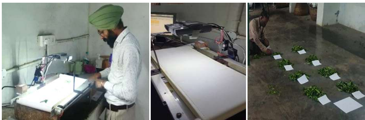
Fig. 1 Scanning of tea leaves using CSIR-CMEERI designed prototype scanning system.
