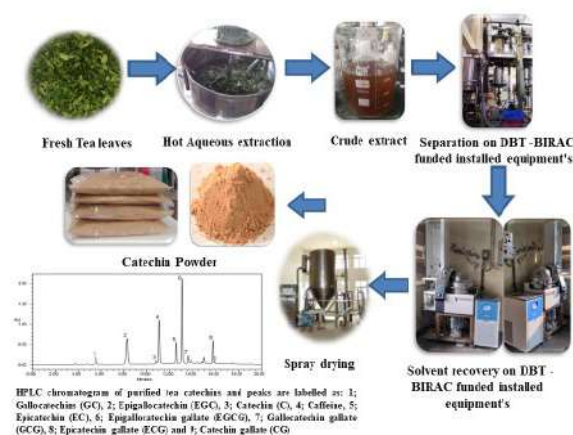
Fig. 5 Processing of green tea leaves @ 50 kg scale for catechin using DBT- BIRAC funded equipment's at CSIR-IHBT Pilot plant.
