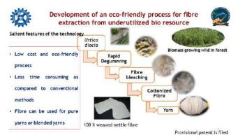
Fig. 1 Process flow for fiber extraction
